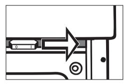
■ To switch the catalyser on, please push the lever located underneath the control panel to the right to position "I".
